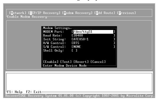
Once you select Enable in the modem initialization popup, the virtual console layout is identical to that of TCP/IP recovery (described above). Additionally, on console [Alt-F5] a modem terminal session is available. By switching to this console and pressing a key, you will be given direct access to the modem.
